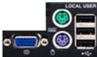
Figure 99: Local User Panel on Dominion KX II
